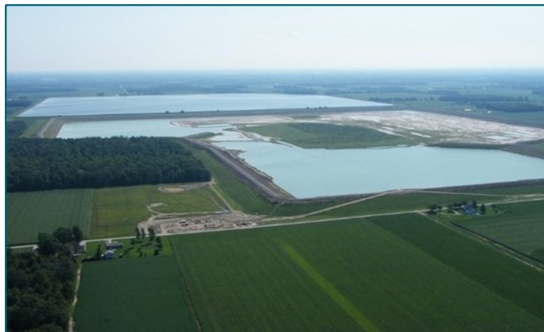
Figure 1: Aerial view of 5.2-billion-gallon Furl Williams Reservoir during construction (Bresler Reservoir is pictured in the background)
