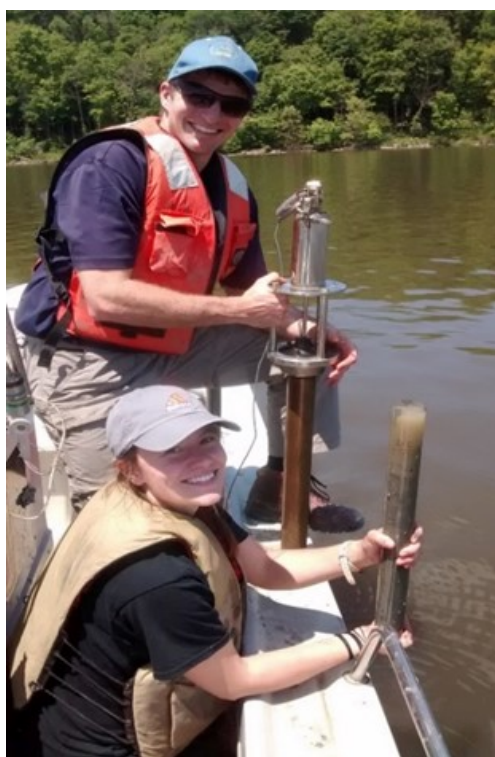
Figure 1. Dr. Jake Beaulieu and Megan Berberich collecting sediment cores with K-B corer
