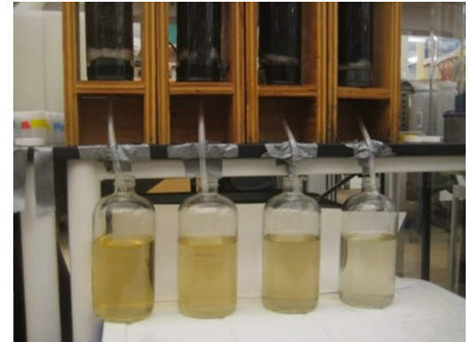
Figure 1. Leachate from laboratory columns of green roof growing media with varying amounts of biochar integrated, ranging from no biochar (left) to high biochar (right). Note the reduction in color due to biochar binding organic matter in the water.
