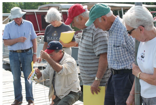
Volunteer training at Charles Mill Lake on May 30 th . Demonstration of Secchi Disk transparency measurement and determination of water color by Pleasant Hill Lakekeeper Steve James.
